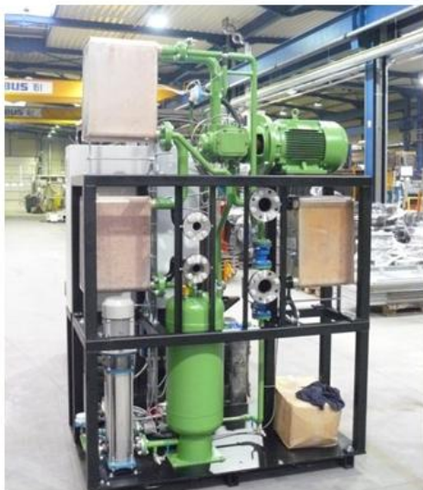
Figure 19 : Heat source, cooling loop, process control and monitoring, 11 kWe ORC
